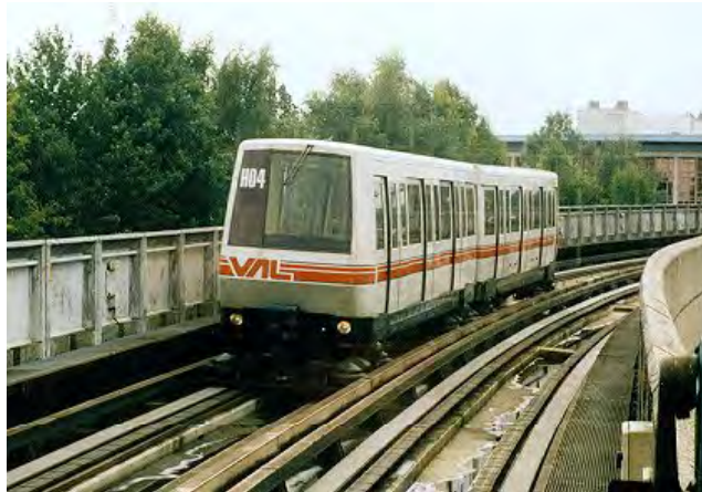
Figure 10-22 Lille VAL (automatic, rubber-tired mini-metro)
