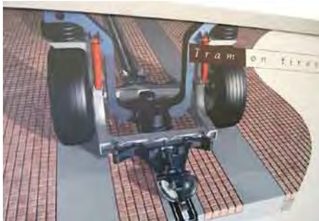
Figure 10-11 Rubber Tyres Guided by Single Steel Rail
