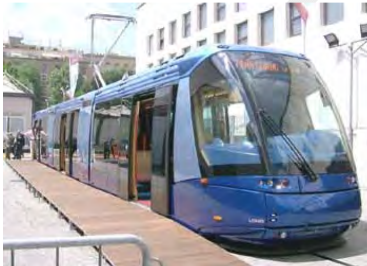
Figure 10-10 Translohr Rubber Tyred Single Rail Tram
