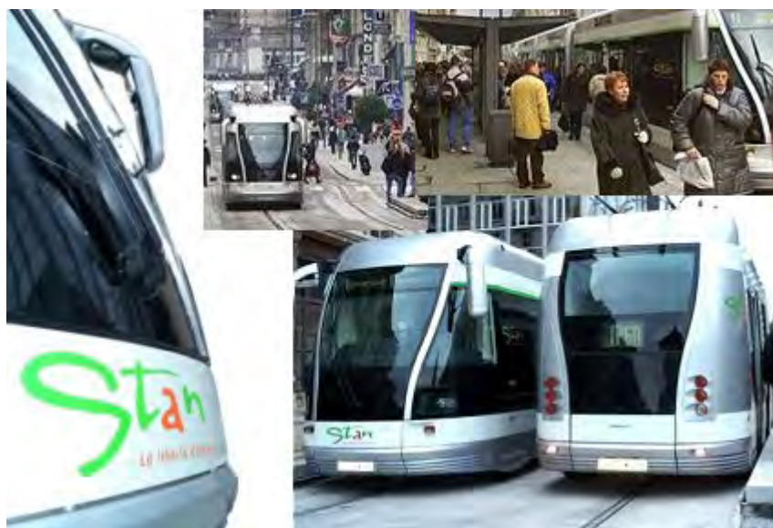
Figure 10-9 GLT (Rubber tyred bus/tram with single rail steering)
